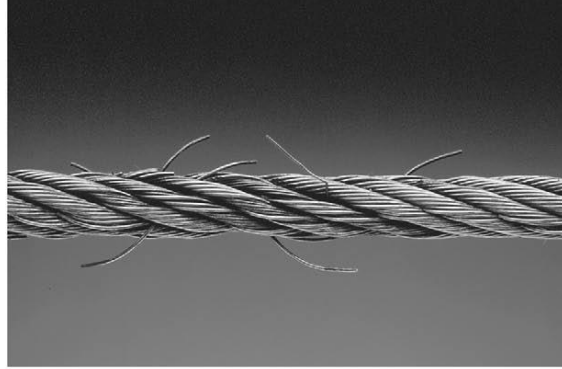
Cable With Broken Wires
